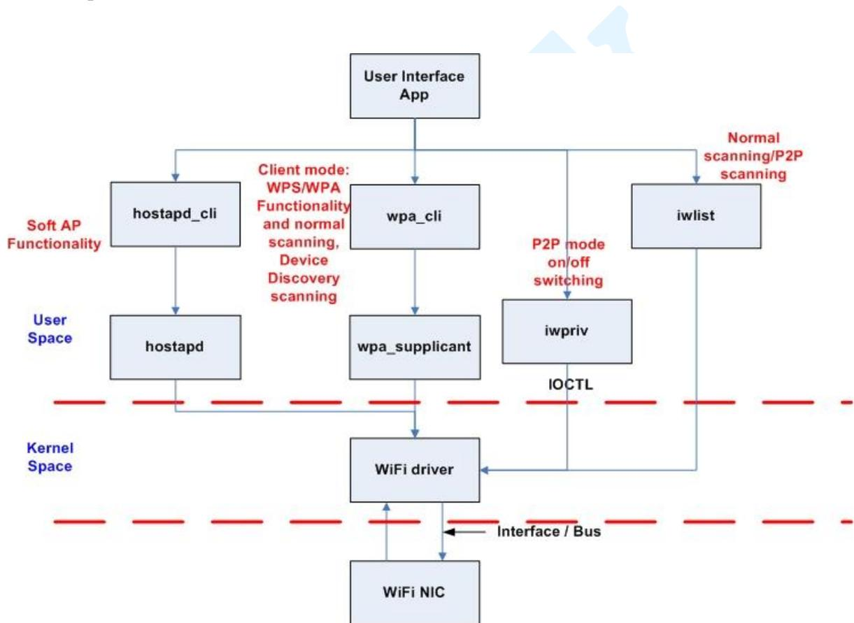
**Figure1: Software Architecture for Realtek Linux Wi-Fi Direct**
