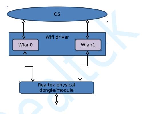
This feature allows performing 2 separate wireless tasks at the same time with single hardware device. For example:
