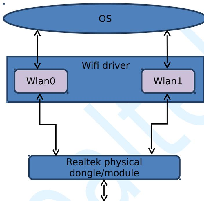
This feature allows performing 2 separate wireless tasks at the same time with single hardware device.
